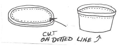
2. Cut the top of the tub off just below the reinforced ring as shown.
